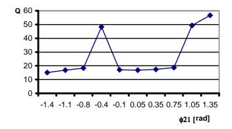
Fig. 4 The correction efficiency Q as a function of the change in the second channel dynamics' coefficient phase shift  $\phi_{21}$ , with other parameters in both channels fixed.
