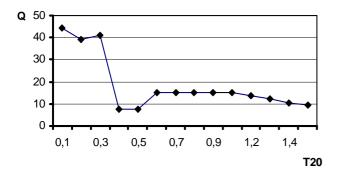
Fig. 2. The correction efficiency Q as a function of a change in the dc component of the dynamics' coefficient  $(T_{20})$  with  $T_{10} = 1.0$
