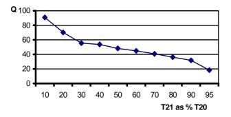
Fig. 3. The correction efficiency Q as a function of a percentage change in the amplitude of the alternate component of the dynamics' coefficient in the second channel (T<sub>21</sub>) with respect to the dc component of this coefficient
