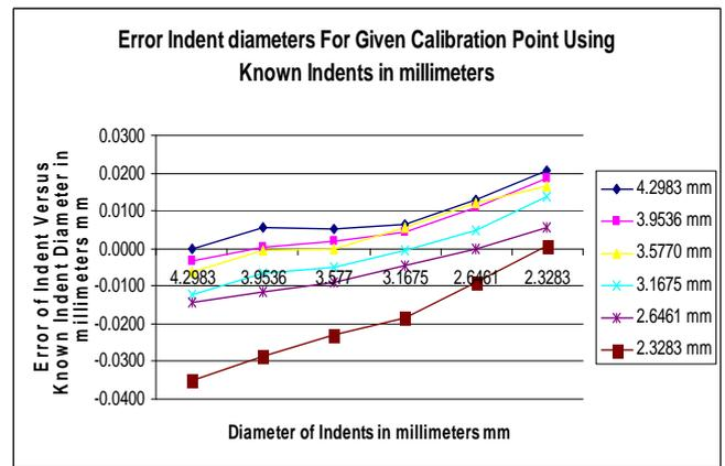
Fig. 5 Image analysis diameter measurements (10 mm ball) after adjustments to known indentation sizes from national laboratories
