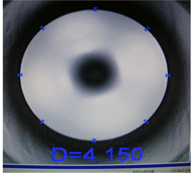
Fig. 2 Brinell indentation measured by image analysis
