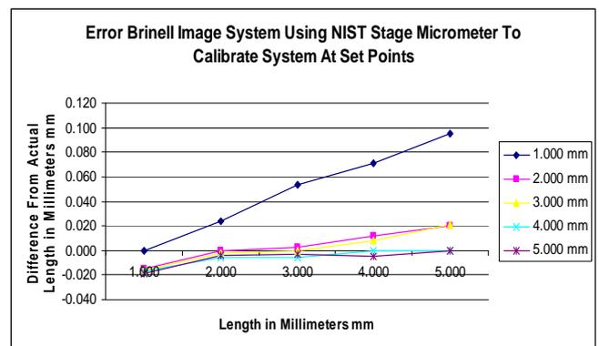
Fig. 7 Image analysis length measurements after adjustment to various points on a stage micrometer from a national laboratory
