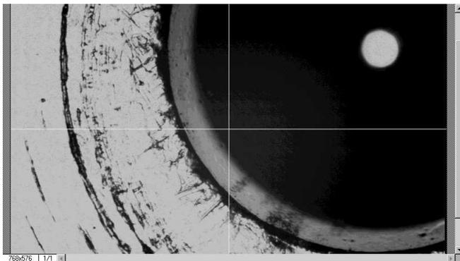
Fig. 1 Brinell indentation shown by NPL microscope
