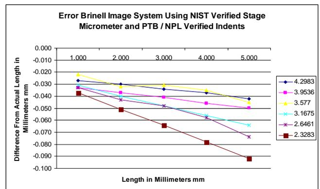
Fig. 6 Image analysis diameter measurements after adjustment to a stage micrometer from a national laboratory
