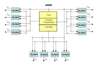
Fig. 1. The connectionist system topology: twelve soft sensors of Elman type to measure contact temperature, humidity and air temperature in four locations of a monument (labels 1-4 correspond to the 4 locations).
