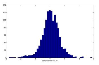
Fig. 5. Histogram of the standard deviations for the substitution error (for temperature  $T_{a1}$ ) for the mixture sensor  $M_{(Q,P,U)}$  providing the best performances in Table 1.
