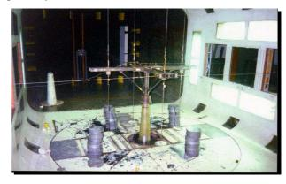
Figure 1. Loading system for balance calibration at TA-2 facility
