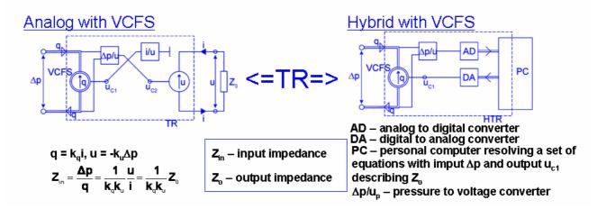
Fig. 2. Transformer - impedance electro-fluidic proportional converter .
