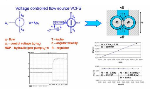
Fig. 3. Electrically controlled flow source FCFS
