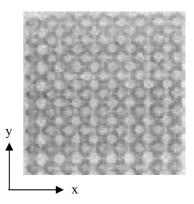
Fig. 6. Image of the MFD of a meander flat coil 50 x 50 mm, number measured samples 128 x 128. Actual image of this specimen was associated with 75 x 75 pixels.
