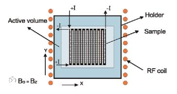
Fig. 2. Orientation of the RF coil, active measuring volume (holder – phantom) and sample in the magnetic resonance imager.
