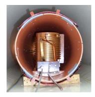
Fig. 3. RF coil located into the magnetic field of a magnetic resonance imager. A cylinder around RF coil represents a gradient coil system designed special for this experiment.
