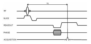
Fig.5. Simplified time diagram of the NMR sequence of the gradient echo.
