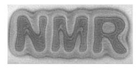
Fig. 8. Image of letters "NMR", dimension 55x17 mm, 512x512 samples
