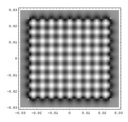
Fig. 4. Density plot of magnetic field for y = 0 for plot points = 75, coil layer (meander): 50 x 50 mm, 19 wires in every layer.
