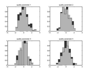
Figure 3. Histograms of four quality parameters, (laboratory analysis, black) and estimated quality parameters (from laboratory analyzer, grey).
