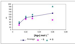
Fig. 4 Chrysene phosphorescence signal in function of the concentration of silver I solution used to spot the substrate (average of measurement  $\pm 1$  Std. Deviation).
