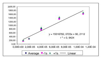
Fig. 8 Analytical curve showing the linear behavior between the chrysene phosphorescence signal in function of the amount of chrysene deposited on substrate (average  $\pm 1$  Std. deviation).
