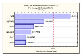
Fig. 6 Pareto's chart showing that it is necessary to refine the model in terms of pH.
