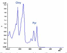
Fig. 10 Absorption spectrum of chrysene (Chry) and pyrene (Pyr)
