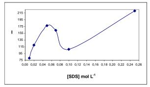
Fig. 5 Silver enhanced chrysene phosphorescence signal in function of the concentration of SDS solution used to spot the substrate (average of measurement  $\pm 1$  Std. Deviation).
