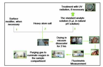
Fig. 2 General procedure for SSRTP
