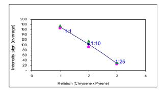
Fig. 9 Effect of increasing amounts of pyrene in the phosphorescence of chrysene (chrysene:pyrene 1:1, 1:10 and 1:25.
