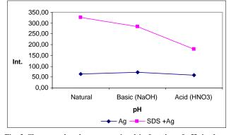
Fig. 3 Chrysene phosphorescence signal in function of pH, in the presence and in the absence of SDS (average of measurement  $\pm 1$  Std. Deviation).
