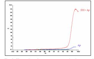
Fig. 3. Silver enhanced room-temperature phosphorescence for chrysene. Natural pH solution in the presence and absence of SDS.
