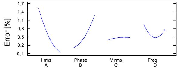
Fig. 4. Main effects for active energy error in sinusoidal conditions
