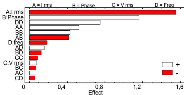
Fig. 3. Pareto chart for active energy error in sinusoidal conditions
