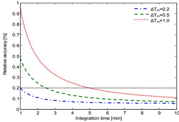
Fig. 2. Accuracy versus integration time
