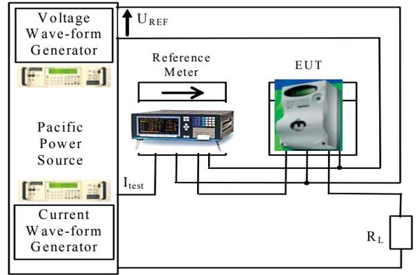
Fig. 1. A block diagram of the performance verification system for single phase energy meters.
