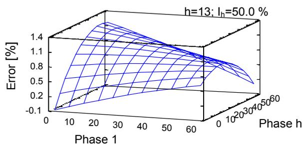
Fig. 15. Estimated response surface for reactive energy error in non-sinusoidal conditions
