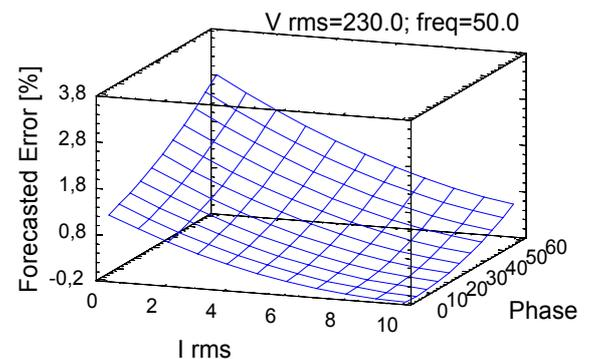
Fig. 6. Estimated response surface for active energy error in sinusoidal conditions
