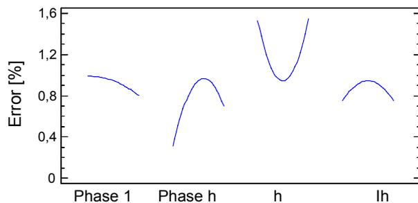
Fig. 13. Main effects for reactive energy error in non-sinusoidal conditions
