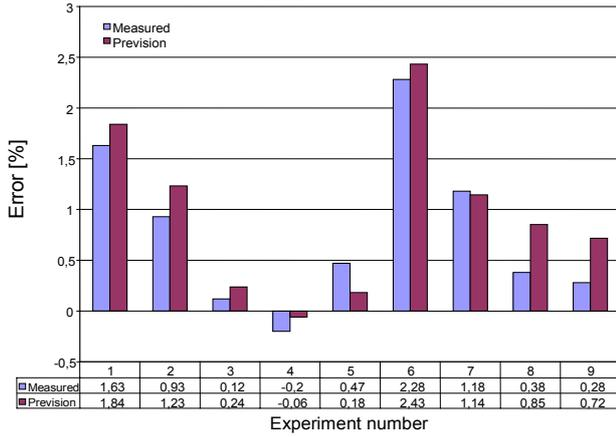
Fig. 7. Forecasting test for active energy error in sinusoidal conditions
