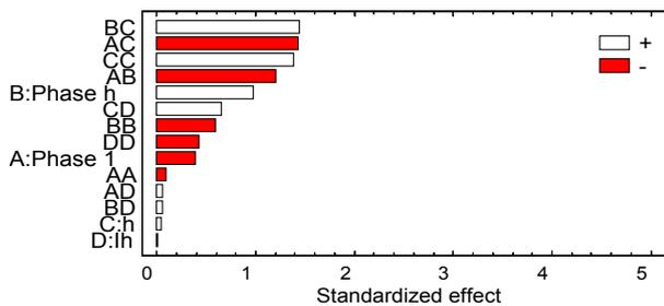
Fig. 12. Pareto chart for reactive energy error in non-sinusoidal conditions
