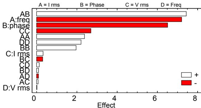
Fig. 8. Pareto chart for reactive energy error in sinusoidal conditions
