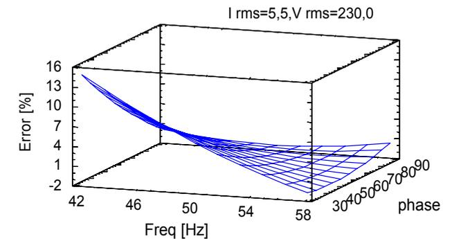
Fig. 11. Estimated response surface for reactive energy error in sinusoidal conditions
