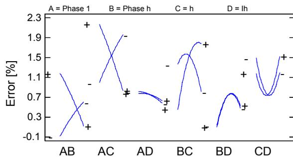
Fig. 14. Interaction plot for reactive energy error in sinusoidal conditions
