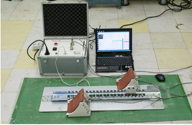
Fig. 5. Measurement equipment of starting block.
