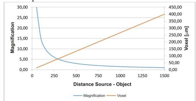
Fig. 4. Magnification and voxel dependency on scanning distance
