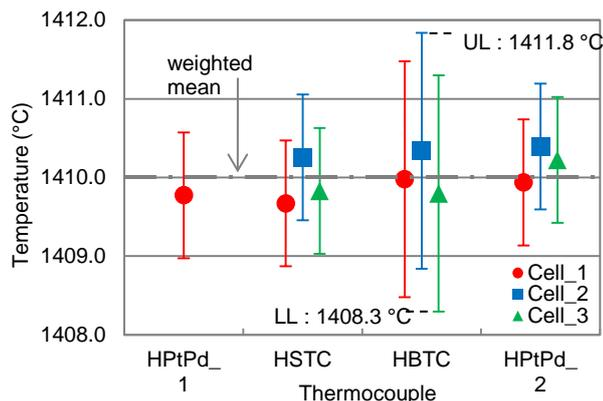
Fig. 3. Summary of the melting temperatures of three Si–SiC cells measured using four thermocouples. The lower limit (LL) and the upper limit (UL) were calculated to be 1408.3 °C and 1411.8 °C, respectively.
