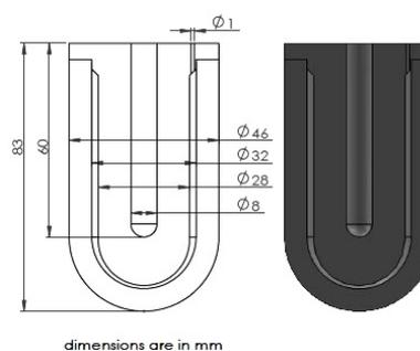
Fig. 1. Schematic drawing and cross-sectional view of the graphite crucible used for the Si–SiC cells.
