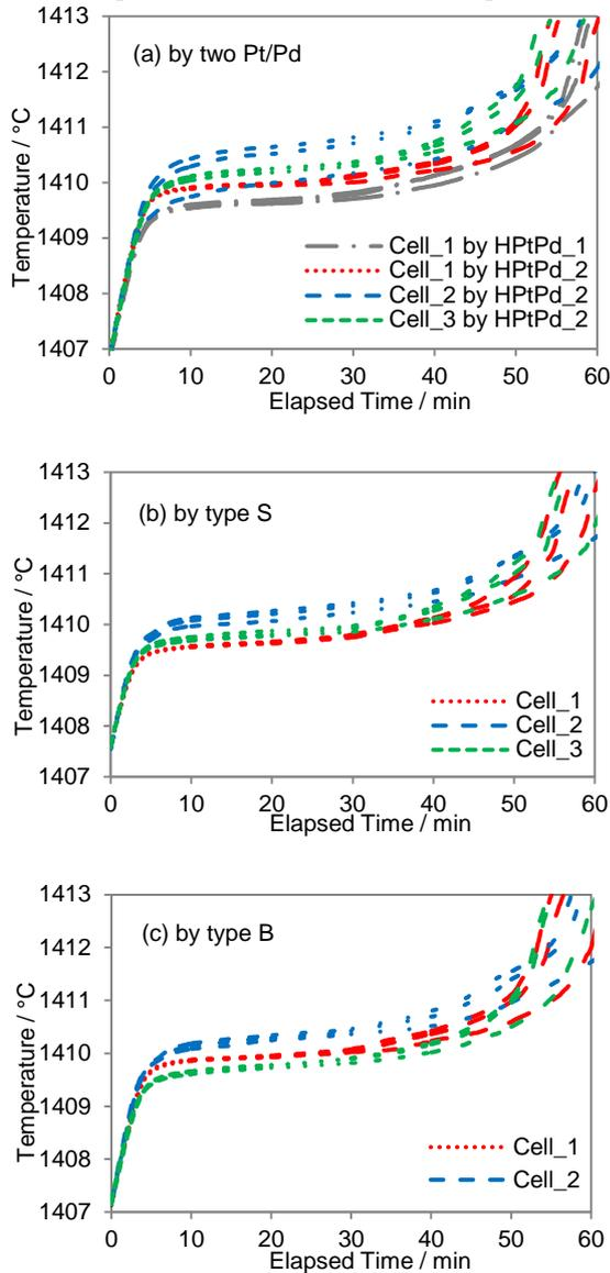
Fig. 2. Melting transitions of the three Si–SiC cells measured using: (a) two Pt/Pd, (b) a type S, and (c) a type B thermocouple. The transition temperature was determined to be 1410.1 °C for the Pt/Pd thermocouples, 1409.9 °C for the type S thermocouple, and 1410.0 °C for the type B thermocouple.
