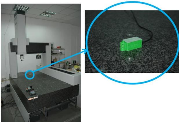
Fig. 4. Digital temperature sensor located in the machine's measuring volume.
