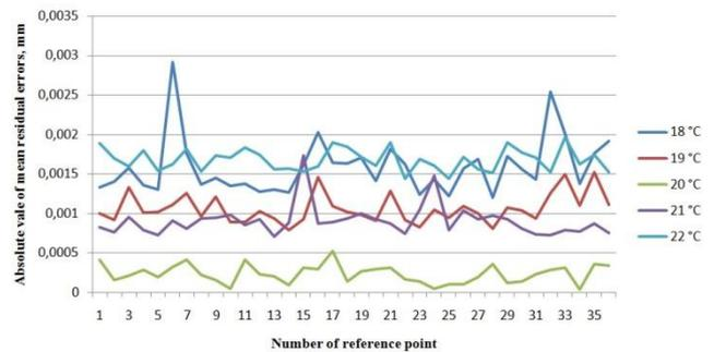
Fig. 3. Absolute values of mean residual errors of coordinate reproduction for z coordinate, determined in different temperatures. Numbers of reference points and their positions are consistent with Tab. 1.
