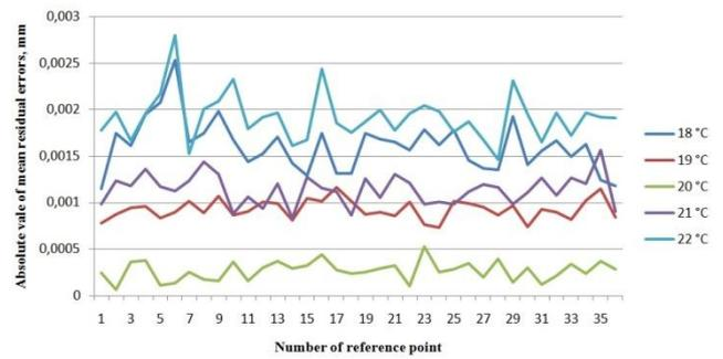
Fig. 2. Absolute values of mean residual errors of coordinate reproduction for y coordinate, determined in different temperatures. Numbers of reference points and their positions are consistent with Tab. 1.
