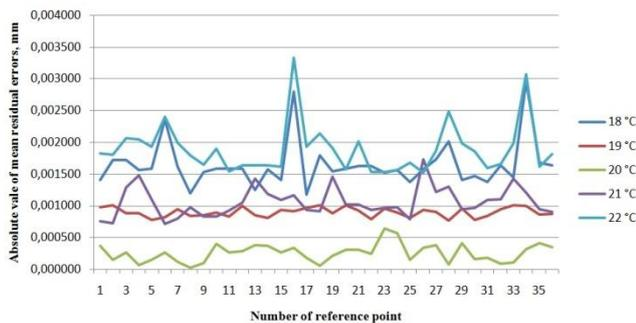
Fig. 1. Absolute values of mean residual errors of coordinate reproduction for x coordinate, determined in different temperatures. Numbers of reference points and their positions are consistent with Tab. 1.
