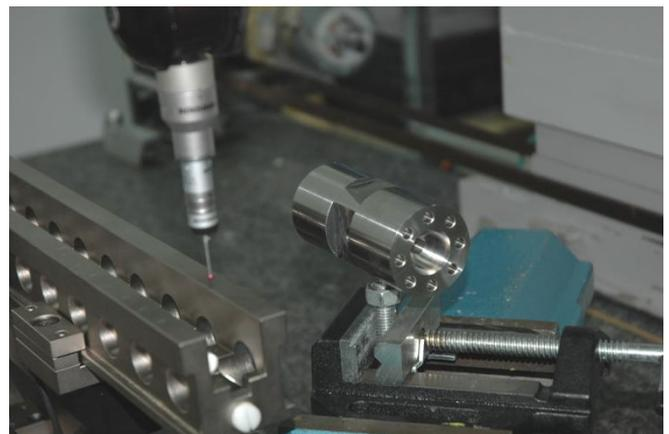
Fig. 5. Verification measurements using multi-feature standard.
