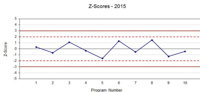
Fig. 7. Control chart indicating performance in control
