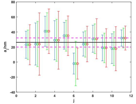
**Fig. 7.** Analysis of key comparison measurement data for a 0.5 mm tungsten carbide gauge block. Uncertainty bars  $x_j \pm 2u_j$ , left,  $x_j \pm \tilde{U}_j$  derived from the posterior predictive distributions, middle, and  $x_j \pm 2\hat{\sigma}u_j$  derived using a Birge adjustment, right. The solid horizontal line indicates the mean and the horizontal dotted lines the 2.5 and 97.5 percentiles of the posterior distribution  $p(\alpha|\mathbf{x})$ .
