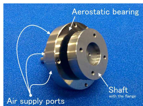
Fig. 8. Photograph of a new aerostatic bearing.
