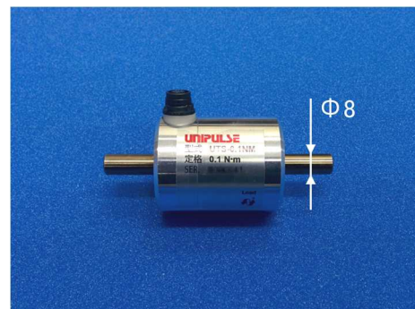
Fig. 7. Photograph of a low nominal capacity TMD.
